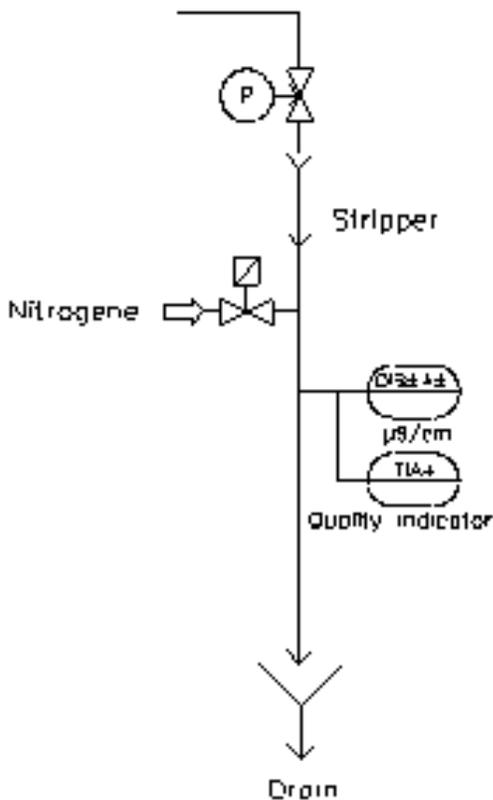
Figure 3. Schematic P+ID of a stripper.
