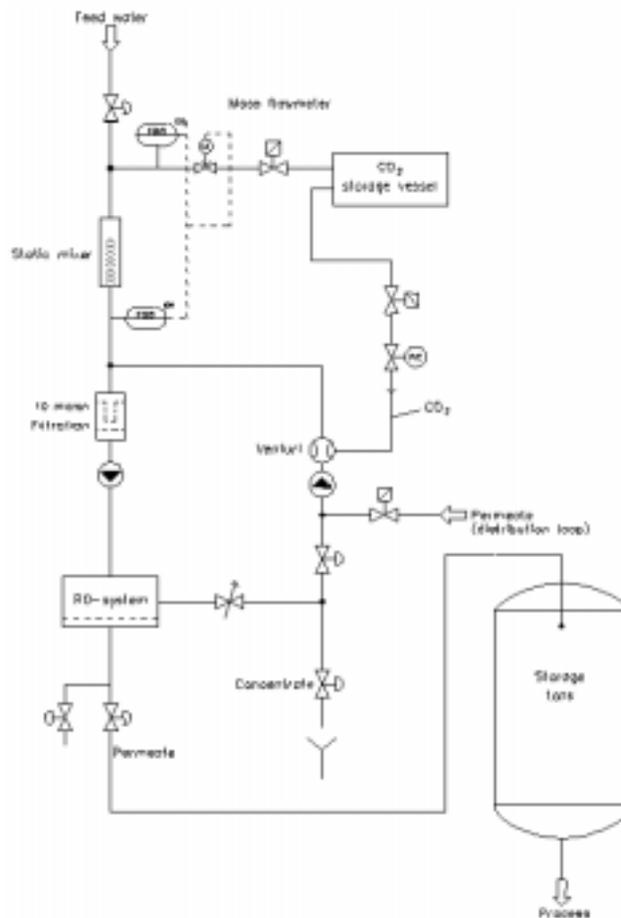
Figure 4. Schematic P + ID of an industrial single-stage RO system for the food industry.
