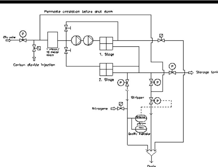
Figure 2. Schematic P+ID of a USP 23 pharmaceutical double-stage RO-system.
